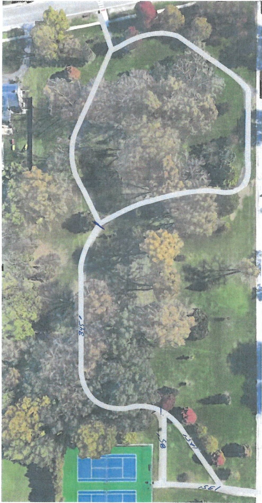
Indian Trails Park, Riegel Road & Willow Road, Homewood Remove and replace marked existing walking trail sections (see photo). Estimated 690', 6' wide in most places. Do your own actual measurement
