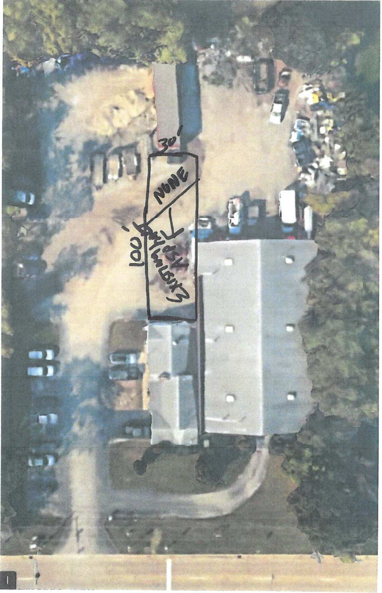
Parks Department, 18900 Kedzie Avenue, Flossmoor. Area to be marked in orange paint. Repair and replace one existing area of asphalt, and add an adjacent section as marked. Total approximately 100' x 30'. Do your own actual measurement
